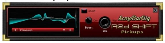
For those of you familiar with Redshift, you'll notice this version is more compact and has a couple different controls. Rather than Volume controls for Wet and Dry, in keeping with the "simple to use theme", we condensed that into one mix knob. Now you can mix your wet and dry signals with one knob. We've added another cool twist, we have made Redshift into an Overdrive box, but be careful, it will drive the heads like crazy.
