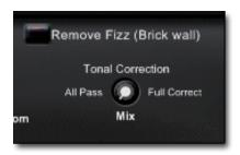
Computer Guitar Amps used at High gain. All Computer Guitar amp models get Fizz in varying degrees at High Gain. One of the techniques employed to remove Fizz is to apply a Low pass filter to your guitar. The Brick Wall Fizz removal control will apply a Low pass filter thus removing Fizz.
